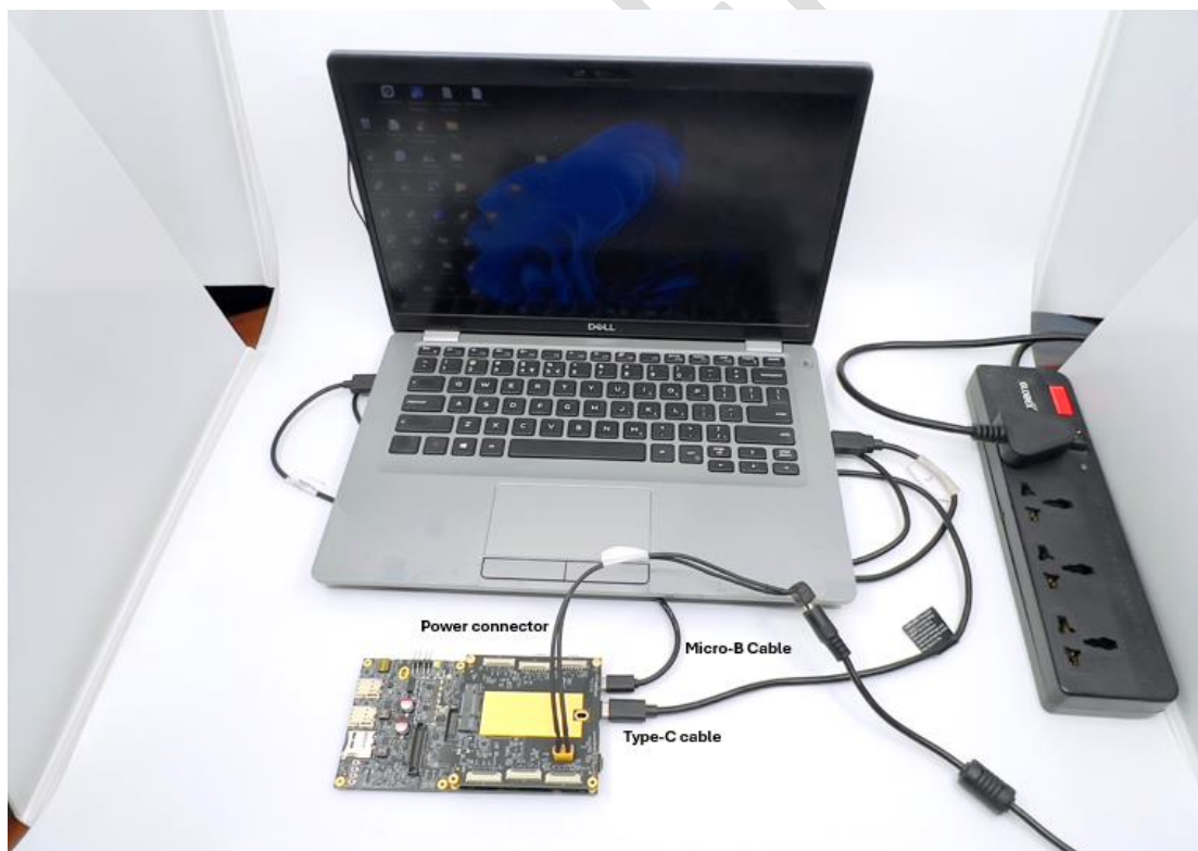
Figure 2: MRD8550 Merlin Kit to Host PC connection
